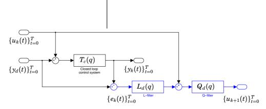
**Figure 2** ILC setup: The update of the correction signal sequence  $\{u_{k+1}\}$  is made in batch after each run.
