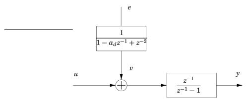
**Figure 3** A blockdiagram of the process. The signal e is white noise and u is the control signal.
