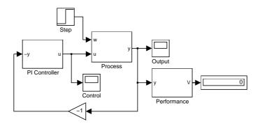
Figure 8 Structure of the Simulink file system\_sim.
