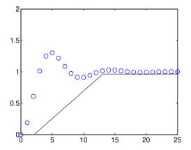
The step response depends linearly on  $Q_k$ , so every time  $t_k$  with a lower bound gives a linear constraint.
