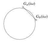
An lower bound  $|G(i\omega_i)|$  is a **nonconvex** quadratic constraint. This should be avoided in optimization.
