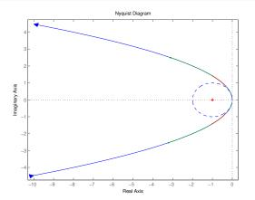
The distance from the loop gain  $L(i\omega I-A)^{-1}B$  to -1 is never smaller than 1. This is always true(!) when  $Q_1>0$ ,  $Q_{12}=0$  and  $Q_2>0$  is scalar. The phase margin is at least  $60^\circ$  and the gain margin is infinite!
