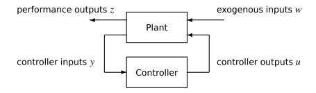
General objective: find a controller that optimizes the closed-loop system  $G_{zw}(s)$ .
