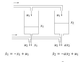
Controllability Gramian:  $W_c = \int_0^\infty \begin{bmatrix} e^{-t} \\ e^{-at} \end{bmatrix} \begin{bmatrix} e^{-t} \\ e^{-at} \end{bmatrix}^T dt = \begin{bmatrix} \frac{1}{2} & \frac{1}{a+1} \\ \frac{1}{a+1} & \frac{1}{2a} \end{bmatrix}$
