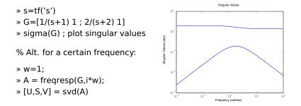
The largest singular value of  $G(i\omega) = \begin{bmatrix} \frac{1}{i\omega+1} & 1\\ \frac{2}{i\omega+2} & 1 \end{bmatrix}$  is fairly constant. This is due to the second input. The first input makes it possible to control the difference between the two tanks, but mainly near  $\omega = 1$  where the dynamics make a difference.
