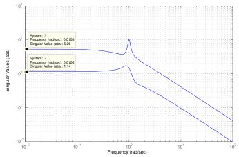
The singular values of the tranfer function matrix (prev slide). Note that G(0)= [2 4 ; 0 3] which corresponds to A in the SVD-example above.  $||G||_{\infty} = 10.3577.$
