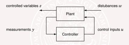
The objective is to find a controller that optimizes the transfer matrix  $G_{zw}(s)$  from disturbances w to controlled outputs z.
