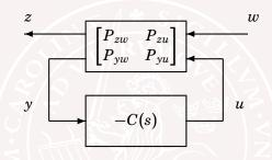
The closed-loop transfer matrix from w to z is
