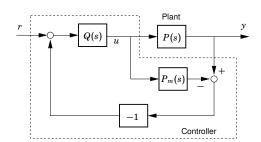
Feedback is used only if the real plant P(s) deviates from the model  $P_m(s)$ . Q(s), P(s),  $P_m(s)$  must be stable.
