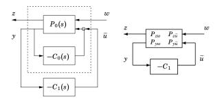
If  $P_0(s)$  is unstable, let  $C_0(s)$  be some stabilizing controller. Then the previous argument can be applied with  $P_{zw}$ ,  $P_{z\widetilde{u}}$ ,  $P_{yw}$ , and  $P_{y\widetilde{u}}$  representing the stabilized system.
