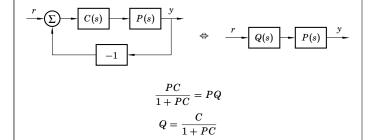
Design Q to get desired closed-loop properties. Then  $C = \frac{Q}{1 - QP}$
