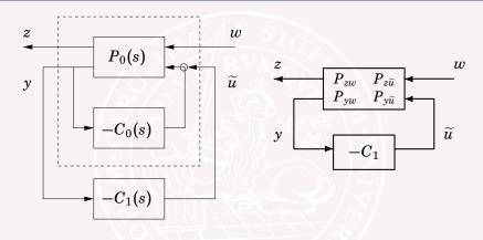
If  $P_0(s)$  is unstable, let  $C_0(s)$  be some stabilizing controller. Then the previous argument can be applied with  $P_{zw}$ ,  $P_{z\widetilde{u}}$ ,  $P_{yw}$ , and  $P_{y\widetilde{u}}$  representing the stabilized system.
