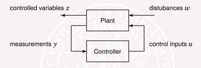
The choice of controller corresponds to designing a transfer matrix Q(s), to get desirable properties of the following map from w to z:
