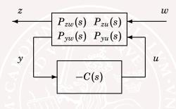
Closed-loop transfer function from w to z:
