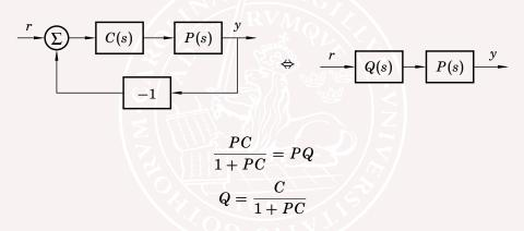
Design Q to get desired closed-loop properties. Then  $C=\displaystyle\frac{Q}{1-QP}$
