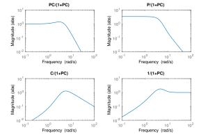
Nonzero static gain in  $\frac{P}{1+PC}$  indicates poor low-freq. disturbance rejection
