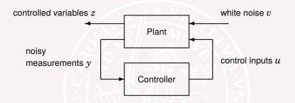
For a linear plant, let v be white noise of intensity R. Find a controller that minimizes the output variance
