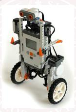
Sensors: Accelerometer, gyroscope
