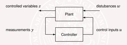
The objective is to find a controller that optimizes the transfer matrix  $G_{zw}(s)$  from disturbances (and setpoints) w to controlled outputs z.
