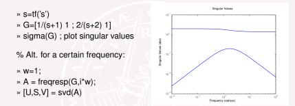
The largest singular value of  $G(i\omega) = \begin{bmatrix} \frac{1}{i\omega+1} & 1\\ \frac{2}{i\omega+2} & 1 \end{bmatrix}$  is fairly constant. This is due to the second input. The first input makes it possible to control the difference between the two tanks, but mainly near  $\omega = 1$  where the dynamics make a difference.
