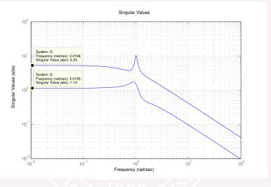
The singular values of the tranfer function matrix (prev slide). Note that G(0)= [2 4 ; 0 3] which corresponds to A in the SVD-example above.  $\|G\|_{\infty}=10.3577.$
