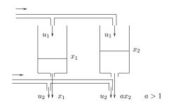
$$\begin{aligned} \dot{x}_1 &= -x_1 + u_1 \\ \dot{x}_2 &= -ax_2 + u_1 \end{aligned}$$
