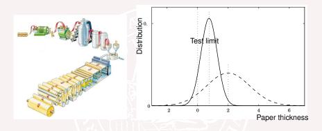
All paper production below the test limit is wasted. Good control allows for lower setpoint with the same waste. The average thickness is lower, which saves significant costs.
