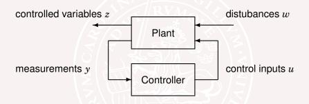
For a linear plant, minimize a quadratic function of the map from disturbance w to controlled variable z
