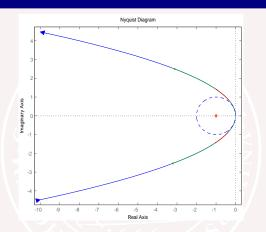
Notice that the distance from  $L(i\omega I-A)^{-1}B$  to -1 is never smaller than 1. This is always true(!) for linear quadratic optimal state feedback when  $Q_1>0$ ,  $Q_{12}=0$  and  $Q_2=\rho>0$  is scalar. Hence the phase margin is at least  $60^\circ$ .
