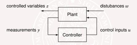
The objective is to find a controller that optimizes the transfer matrix  $G_{zw}(s)$  from disturbances w to controlled outputs z.
