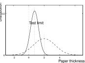
All paper production below the test limit is wasted. Good control allows for lower setpoint with the same waste. The average thickness is lower, which saves significant costs.
