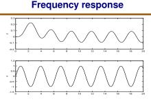
The transfer function G(s) is the Laplace transform of the impulse response  $G = \mathcal{L}g$ . The input  $u(t) = \sin \omega t$  gives
