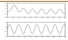
The transfer function G(s) is the Laplace transform of the impulse response  $G=\pounds g$ . The input  $u(t)=\sin\omega t$  gives
