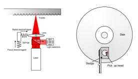
The pick-up-head has two electromagnets for fast positioning of the lens (left). Larger radial movements are taken care of by the sledge (right).
