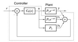
Idea: Make an internal model of the process (with and without the delay) in the controller. Ideally Y and  $Y_1$  cancel each other and use feedback from  $Y_2$  "without delay".
