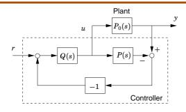
Feedback is used only as the real process deviates from P(s).
