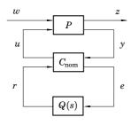
where  $C_{\text{nom}}$  stabilizes the [P, C]-system and Q(s) is any stable transfer function.
