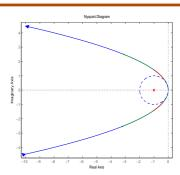
Notice that the distance from  $L(i\omega I-A)^{-1}B$  to -1 is never smaller than 1. This is always true(!) for linear quadratic optimal state feedback when  $Q_1>0$ ,  $Q_{12}=0$  and  $Q_2=\rho>0$  is scalar. Hence the phase margin is at least  $60^\circ.$
