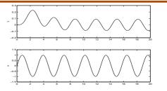
The transfer function G(s) is the Laplace transform of the impulse response  $G = \pounds g$ . The input  $u(t) = \sin \omega t$  gives
