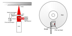
The pick-up-head has two electromagnets for fast positioning of the lens (left). Larger radial movements are taken care of by the sledge (right).
