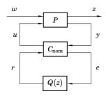
where  $C_{nom}$  stabilizes the [P,C]-system and Q(z) is any stable transfer function.
