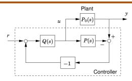
Feedback is used only as the real process deviates from P(s). The transfer function Q(s) defines how the desired input depends on the reference signal.
