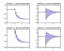
A Kalman filter estimates the states using measured positions. Why is the transient error bigger in the right plots?
