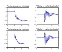
The measurement  $y_2$  is not trusted, so the estimate of  $x_3$  slows down.
