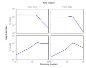
Nonzero static gain in  $\frac{P}{1+PC}$  indicates poor disturbance rejection
