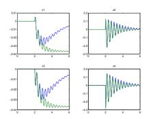
When only velocity is penalized, a static position error remains
