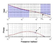
Remark: approximations inexact around cross-over frequency  $\omega_c$ . In this region, focus is on stability margins  $A_m$ ,  $\phi_m$ .
