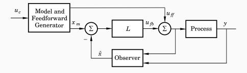
The model should generate a reference trajectory  $x_m$  for the process state x (one reference signal per state variable)
