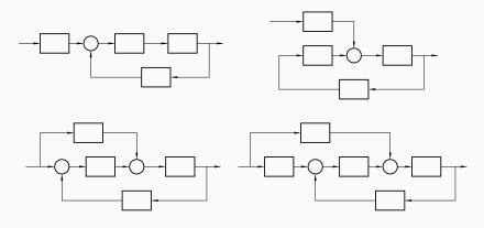
For linear systems, all these structures are equivalent
