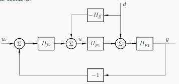
Pulse transfer function from measured disturbance d to output y:
