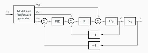
ullet The PID controller should have derivative weighting  $\gamma=1$
