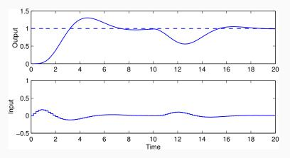
Does not work very well – the feedforward term is needed to get the desired setpoint response
