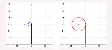
$k_i = \omega_c = 0.005\omega_0$  (blue), will give stable closed loop  $k_i = \omega_c = 0.02\omega_0$  (red), will give unstable closed loop
