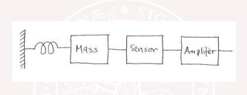
Want the accelerometer to be both sensitive and fast Simple model of an accelerometer without control
