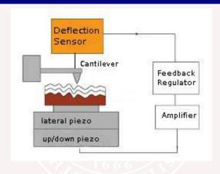
Using an atomic force microscope (AFM) one can measure molecular forces between a fine tip and a surface
