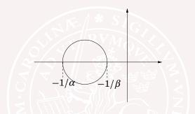
The system (3) with sector condition (2) is absolutely stable if the origin is asymptotically stable for  $\psi(t, y) = \alpha y$  and the Nyquist plot
