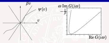
Suppose that  $\psi : \mathbf{R} \to \mathbf{R}$  is Lipschitz and  $0 \le \psi(v)/v \le \beta$ . Let  $G(i\omega) = C(i\omega I - A)^{-1}B$  with A Hurwitz and (A,B,C) minimal. If there exists  $\eta \in \mathbf{R}$  such that
